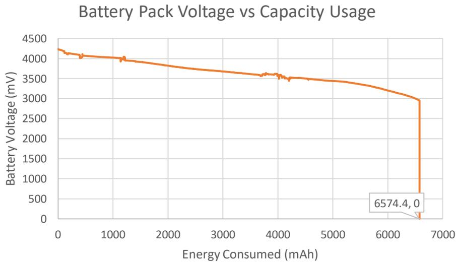
We can see here the measured capacity was 6574mAh – the minor difference (0.3%) when compared to the theoretical value likely being due to accumulated measurement errors.
