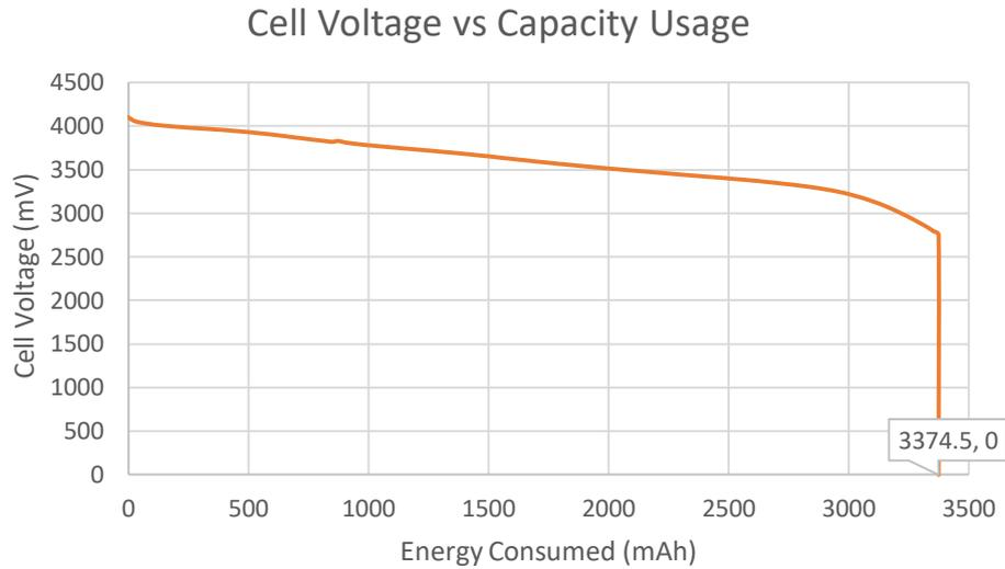
Here we can see the capacity of each cell was measured at 3374.5 mAh (vs 3300mAh rating) – two of these batteries connected in parallel should therefore produce a pack with 6749mAh capacity.
