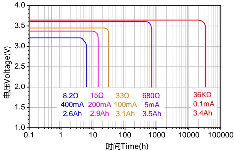
LiSoCl<sub>2</sub> packs are unable to provide the high discharge currents required for cellular connectivity on their own: capacitors are used to smooth out the short power bursts. The net effect is that the devices take an average of 60-90mA during transmission cycles, and 0.04mA during sleep cycles. As such the orange curve (33Ω) is most representative during transmission cycles (~0.3% of device lifetime) and the red curve (36KΩ) most representative of sleep (~99.7% of device life).
